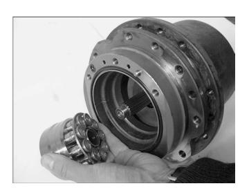
27. Set the motor on its side and fit the cylinder block subassembly using the spline in the shaft as a guide.
