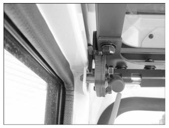
Tuck the front opening window in the ceiling to see if it can be tightly locked.
