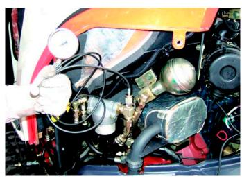
2)Accumulator discharge pressure test.
