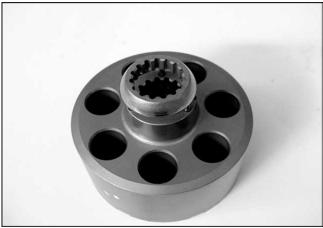
15. Fit the retainer holder to the cylinder barrel.
