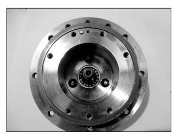
11. Fit the control piston, steel ball and shaft to the body 2.
