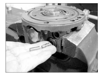
5. Insert the shuttle spool and needle (both sides) in to the body 1.
