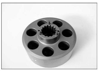
14. Insert the pins (3 pairs) into the cylinder barrel.
