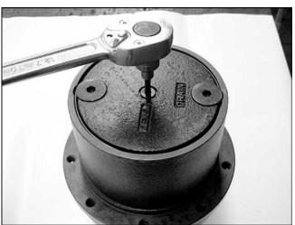
19. Fit the flanged plug (G3/8) to which the O-ring is fitted.
