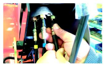
2. While pushing the hose upward, grip down the plastic socket and pull down the hose assy.
