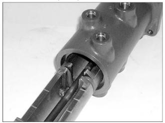
Seal inserting tool Tool No.: KS000-00130
