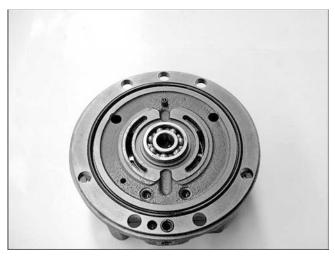
7. Press-fit the bearing and spring pin into the body 1. Then fit the O-rings (2 places).
