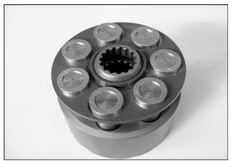
16. Using the shoe holder assembly and barrel holder, assemble the cylinder barrel assembly.
