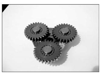
11. Fit the gear b2 and needle to the carrier II in this order.
