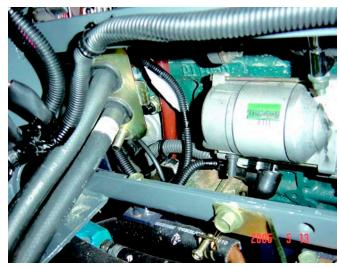
(1) Nut tightening torque for connecting cable to starter terminal 5.9~11.8N⋅m (0.6~1.2kgf⋅m) 4.34~8.68ft⋅lbs
