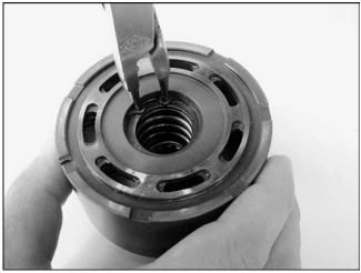
13. Fit the retainer, spring and retainer to the cylinder barrel in this order and fix them with the snap ring.
