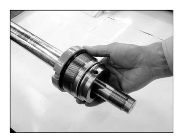
11) Pull out the cylinder head. Release the piston rod from the vise.
