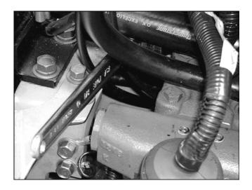
Check the anti-void valve for heavy movement, scratches, foreign matters, etc.
