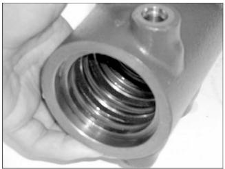
Insert the seal ring using a specific tool.
