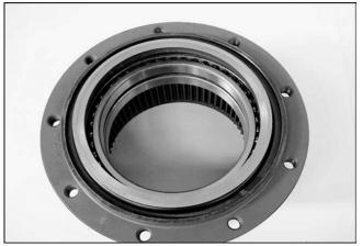
4. Fit the floating seat combined with the O-ring.\* If it is difficult to fit it, apply grease to the O-ring.
