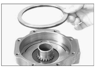
18. Check the inner and outer O-rings of the ring for scratches and distortion, and apply hydraulic oil to them before assembling.
