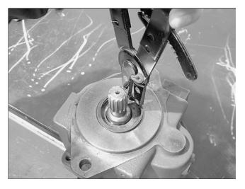
5. Dismounting the oil seal Remove the snap ring (34) provided at the drive shaft (3) from the body S.
