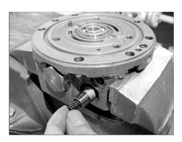
3. Insert the two-speed spool and spring into the body 1.
