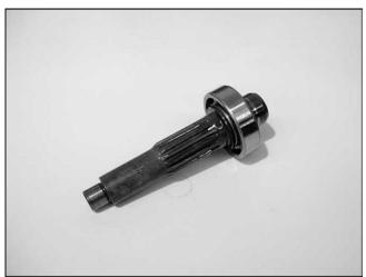
10. Press-fit the bearing onto the shaft.
