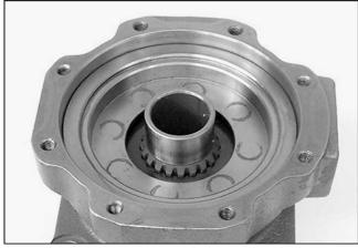
19. Check the outer O-ring of the piston for scratches and distortion, and apply hydraulic oil to it before assembling.
