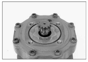
21. Fit the 2 different O-rings into the O-ring grooves of the flange mounting. Insert the drive.
