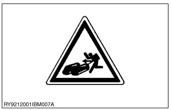
Grease is under high pressure inside the hydraulic cylinder. It is very dangerous to loosen a grease nipple quickly as it may shoot off. Always loosen grease nipples slowly.
