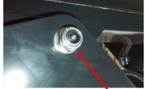
Fix plate pin W21CSH0191 to the external (perforated) plate W21CSH0980
