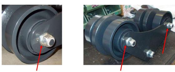
Install washer Ø18 and nut M18 on the rollers
