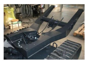
2. Remove the bolts between the body support and the slew ring
