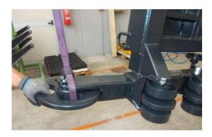
3. Remove wheel screws and bolts
