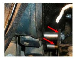
21.Remove the four screws indicated in the pictures below from the engine support
