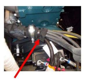
19. Attention: Oil pump is not directly fixed at the chassis. Disconnecting it from the engine, oil pump will remain hanged only by oil tubes; it is necessary to locate a support between the oil pump and the chassis in order to hold it up.
