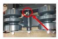
By a grease pump, grease the pin by the greaser. Grease has to come out from the back
