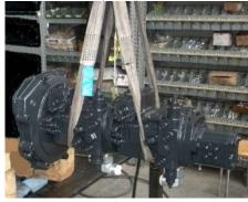
8. In case of difficulties because of the restrict working area, it is possible to remove back gears pump from the pump unit
