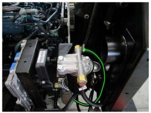
9. Remove the air filter and its pipes
