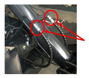
5. Remove the lower cylinder body pin, then remove the cylinder
