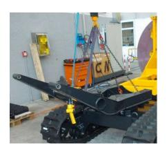
4. Remove the spacer from the slew ring
