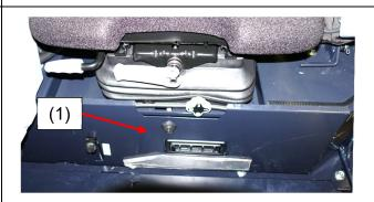
Step 25: Reconnect the hose (1) and the connector (2) to the washer fluid tank.
