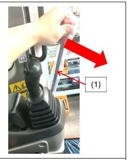
Step 5: Loosen the lock nut (1) of the stopper bolt (2).
