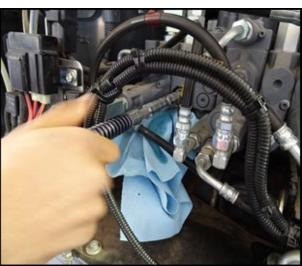
Reassemble the spool cap and reconnect the pilot hose of the left travel section.
