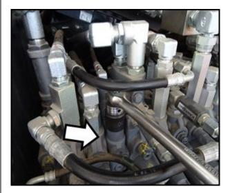
Pull out the spool and the spring seat using the pliers as shown in the figure below.
