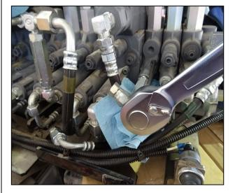
Flush the countermeasure spool and insert it into the swivel section of the valve.
