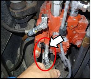
Remove the two orifices of the LS valve as shown in picture below. (Color of orifice: pink, black)
