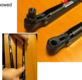
**Step 9 :** Change the wiper arm, left to right and right to left. Press the iron handle inside the wiper arm and push in the wiper lever to the desired length. Repeat this step for the other arm, as shown in below photos.
