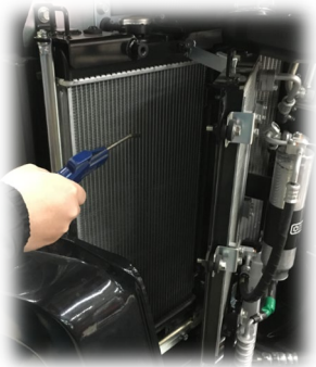
Radiator and oil cooler side by side layout
