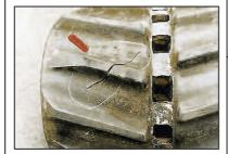
Replace rubber track if the damage is following condition.
