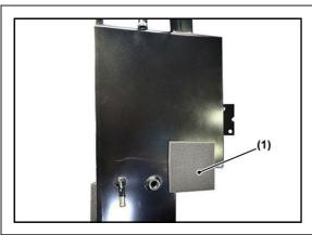
17. Affix the sound absorbing material (1) by aligning it with the bottom right corner on the opposite face of the oil level gauge face.
