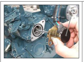
1. Remove the engine stop solenoid (1) according to the engine WSM.
