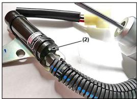
1. Install the new engine stop solenoid (1) according to the engine WSM.
